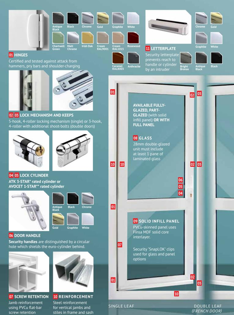
\*ATK 3-STAR cylinder can be used with our **standard** door handle to achieve Secured by Design, \*\*Avocet 1-STAR cylinder must be used with our **security** door handle to achieve Secured by Design
